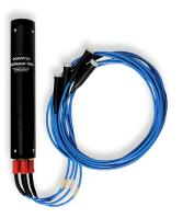
The AQUA*scat*® 1000R is an acoustic suspended sediment profiler specially designed and manufactured as a research model. 4 cabled transducers are supplied with the instrument, each of which transmits short pulses of ultrasound, which are then scattered back by the sediment in the
