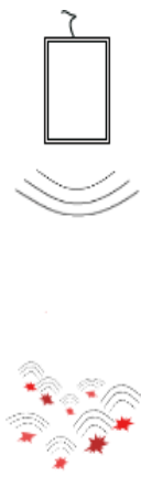
Figure 1: Acoustic backscatter principle
