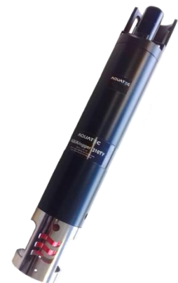
Figure 2: AQUAlogger 310TY – self-contained turbidity logger
