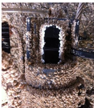
Figure 3: Biofouling on an AQUAlogger 210TY – optical window cleaned by mechanical wiper (image courtesy of Fugro EMU)
